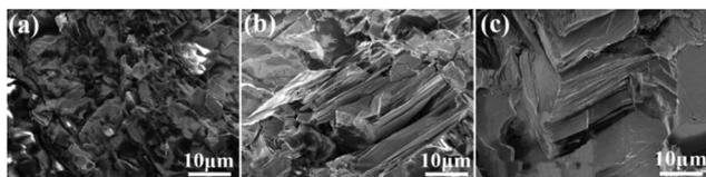
**Fig. 2** The SEM image of the fractured surfaces parallel to the pressure direction for the  $\text{Na}_{0.03}\text{Sn}_{0.97}\text{Se}-x\%\text{Te}$  samples with (a)  $x = 0$ , (b)  $x = 5$ , and (c)  $x = 15$ .
