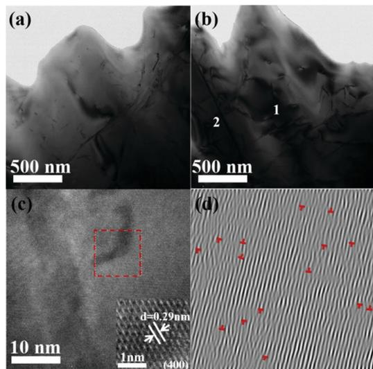
Fig. 5 Microstructure of the LPHD samples: (a) low-magnification TEM image of  $\text{Na}_{0.03}\text{Sn}_{0.97}\text{Se}-0\%\text{Te}$ ; (b) low-magnification TEM image of  $\text{Na}_{0.03}\text{Sn}_{0.97}\text{Se}-5\%\text{Te}$  with the defects in the matrix; (c) HRTEM image from (b) the region marked 1 with the FFT image and its interplanar spacing; (d) inverse FFT image of the red box in panel (c) obtained from the (400) reflection.
