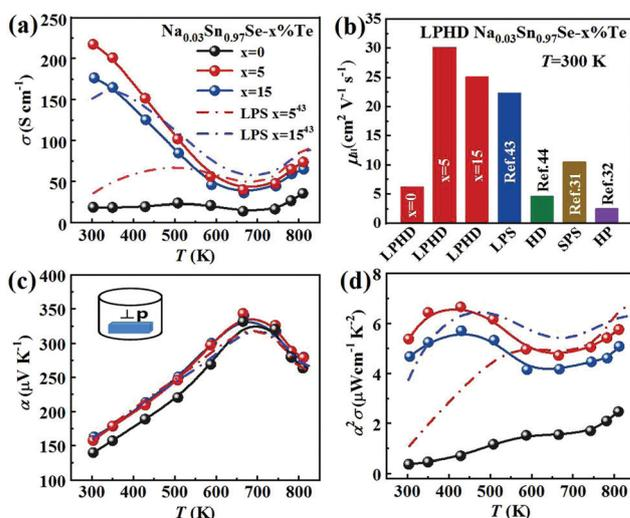
**Fig. 3** Temperature dependence of  $\text{Na}_{0.03}\text{Sn}_{0.97}\text{Se}-x\%\text{Te}$  ( $x = 0, 5$  and 15) LPHD samples: (a) electrical conductivity, (b) room temperature Hall mobility with some previous reports as a comparison, (c) Seebeck coefficient and (d) power factor.
