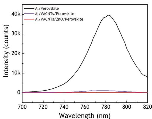
Fig. 5 Steady-state photoluminescence spectroscopy (exc. 470 nm) of Al/perovskite, Al/VACNT/perovskite, and Al/VACNT/ZnO/perovskite samples.
