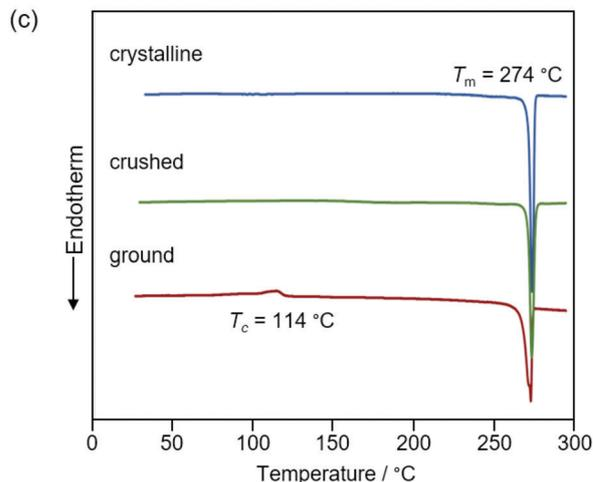
**Fig. 10** (a) Photographs for the two-step MCL of **1g** excited with UV light (365 nm). (b) PXRD patterns for the crystalline (blue), crushed (green), ground (red), and heated (purple) samples of **1g**. (c) DSC scans for the crystalline (blue), crushed (green), and ground (red) samples of **1g**.  $T_m$  and  $T_c$  values are noted near the corresponding peaks.
