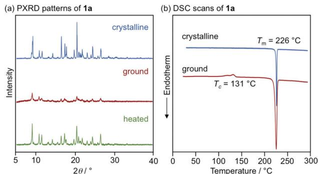
Fig. 8 (a) PXRD patterns for the powdered crystalline (blue), ground (red), and heated (green) samples of **1a**. (b) DSC scans for crystalline (blue) and ground (red) samples of **1a**.  $T_{\text{m}}$  and  $T_{\text{c}}$  values are noted near the corresponding peaks.
