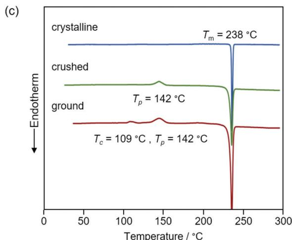
**Fig. 9** (a) Photographs for the two-step MCL of **1e** excited with UV light (365 nm). (b) PXRD patterns for the crystalline (blue), crushed (green), ground (red), and heated (120 °C, purple and 180 °C, orange) samples of **1e**. (c) DSC scans for the crystalline (blue), crushed (green), and ground (red) samples of **1e**.  $T_m$ ,  $T_p$ , and  $T_c$  values are noted near the corresponding peaks.
