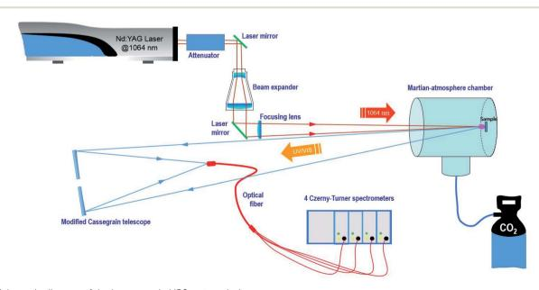
Fig. 1 Schematic diagram of the home-made LIBS system design.
