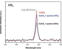
Fig. 4 Emission intensity of the atomic carbon signal from both the pure  $CaCO_3$  matrix and that doped with 10% pyrene in both air and the  $CO_2$  atmosphere.
