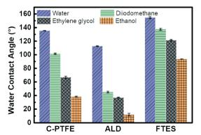
Fig. 4 Water and low surface tension liquid (diiodomethane, ethylene glycol and ethanol) contact angles of C-PTFE and ALD and FTES modified membranes. Error bars indicate the standard deviation of three repeated measurements from two membrane samples.
