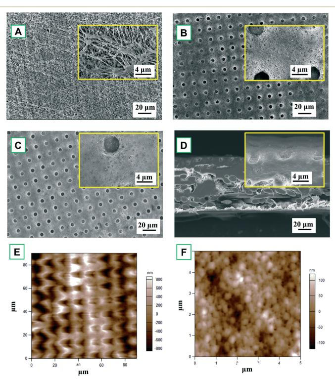
Fig. 2 SEM images of the membrane surface: (A) pristine PTFE (C-PTFE); (B) TiO<sub>2</sub> atomic layer deposited nanoimprinted membrane (ALD); (C) fluorinated ALD membrane (FTES); (D) cross-section of FTES. Atomic force microscopy (AFM) images of (E) the membrane surface demonstrating the dot pattern and (F) deposition layer of TiO<sub>2</sub>.
