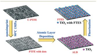
Fig. 1 Schematic illustration of design and procedures for fabricating the nanoimprint PTFE membrane with a fluorinated TiO2
