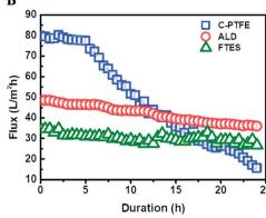
Fig. 5 Comparison of the filtration performance of C-PTFE and ALD and FTES modified membranes: (A) permeate conductivity and (B) water flux.
