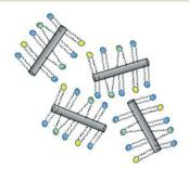
Fig. 3 Predicted mode of adsorption of phospholipids to the walls of SWCNT  $\it via$  the acyl chains, as determined by molecular docking simulations.  $^{65}$
