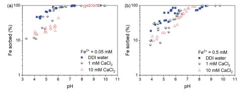
Fig. 1 Percentage of Fe<sup>2+</sup> sorbed on Syn-1 ( $\sim$ 1 g L<sup>-1</sup>) as a function of pH at different CaCl<sub>2</sub> concentrations. Samples in DDI water had a Ca<sup>2+</sup> concentration of  $\sim$ 0.1 mM after 1 day equilibration. Total Fe<sup>2+</sup> concentrations of (a) 0.05 and (b) 0.5 mM were added and equilibrated for 1 day with 1 g L<sup>-1</sup> Syn-1.
