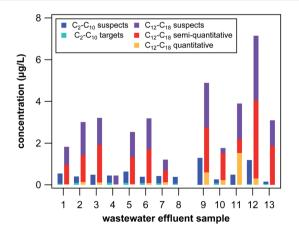
Fig. 2 Approximate total concentrations of QACs with side-chains of 10 or less C atoms (left-side bar) and QACs with side-chains of 12 and more C atoms (right-side bar) in all 13 effluent samples. Total bar height indicates the sum of all target and suspect QACs for each group. Bars are color-coded for the amounts contributed by quantitative targets (bottom part, teal and orange), semi-quantitative targets (middle part, red, right bars only), and suspects (top part, blue and purple).
