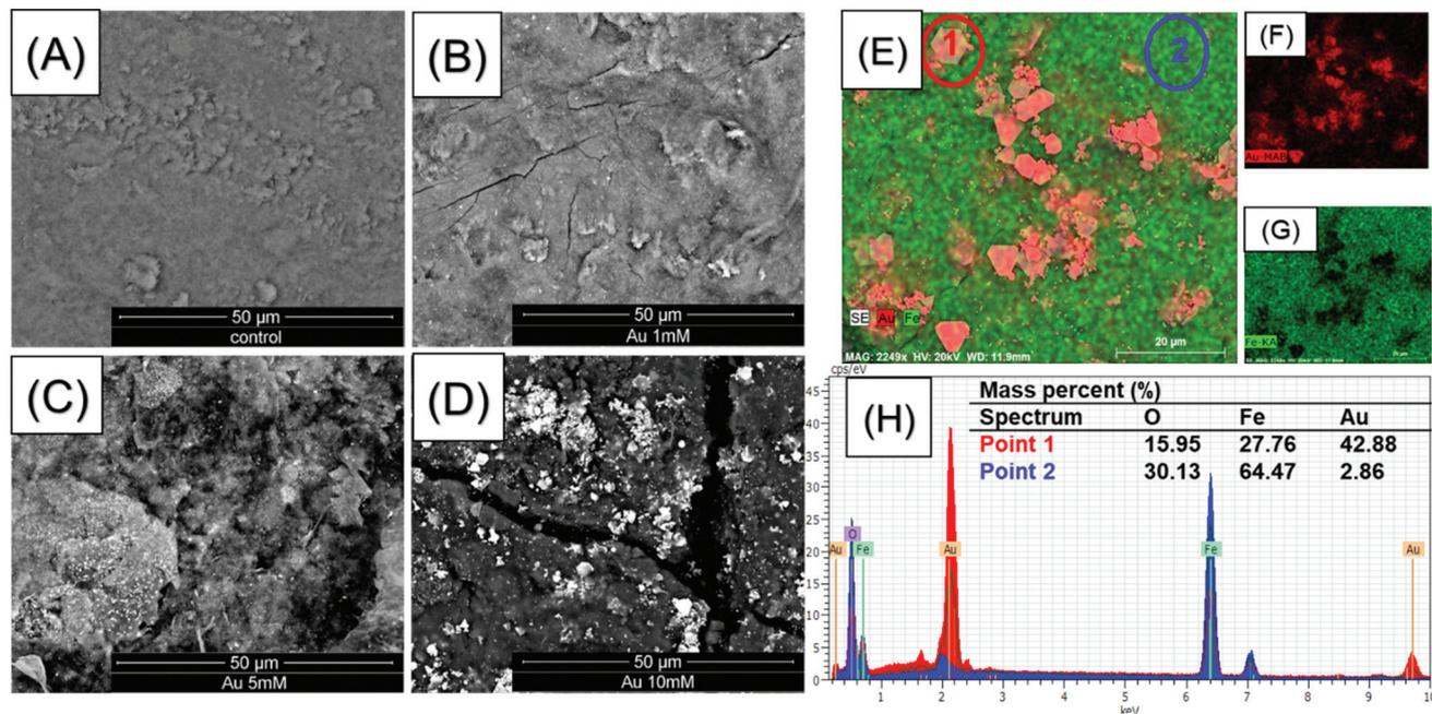
**Fig. 2** Backscattered SEM images of the aggregated (A) Fe<sub>3</sub>O<sub>4</sub>@BCNCs, (B) 1 mM Au@Fe<sub>3</sub>O<sub>4</sub>@BCNCs, (C) 5 mM Au@Fe<sub>3</sub>O<sub>4</sub>@BCNCs and (D) 10 mM Au@Fe<sub>3</sub>O<sub>4</sub>@BCNCs. EDS mapping of (E) 10 mM Au@Fe<sub>3</sub>O<sub>4</sub>@BCNCs with (F) Au and (G) Fe elements highlighted. The corresponding (H) EDS spectra of the map are provided with mass percent of O, Fe, and Au shown.
