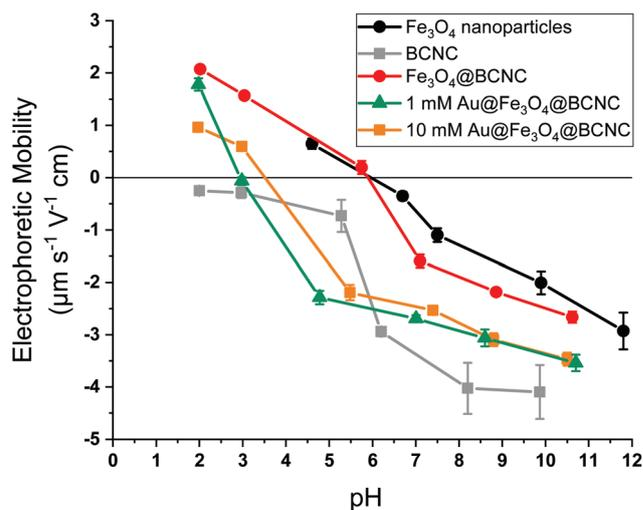
**Fig. 3** Electrophoretic mobility of bare Fe<sub>3</sub>O<sub>4</sub> nanoparticles, BCNCs, Fe<sub>3</sub>O<sub>4</sub>@BCNCs, 1 mM and 10 mM Au@Fe<sub>3</sub>O<sub>4</sub>@BCNCs in 0.01 M NaCl solution. The error bars indicate standard deviation of three measurements.
