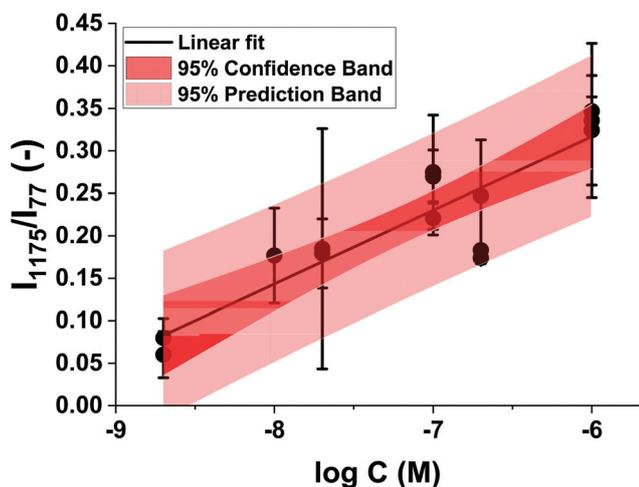
Fig. 6 The comprehensive plot of the normalized Raman peak of 1175 cm<sup>-1</sup> vs. the logarithm of the concentrations of MGITC using 1, 5, and 10 mM Au@Fe<sub>3</sub>O<sub>4</sub>@BCNCs. The black solid line shows the best-fit linear curve. Dark and light red-colored regions show statistical 95% confidence and prediction bands, respectively.  $R^2 = 0.79$ , Linear fit:  $I_{1175}/I_{77} = 0.837 + 0.087 \log C$ .
