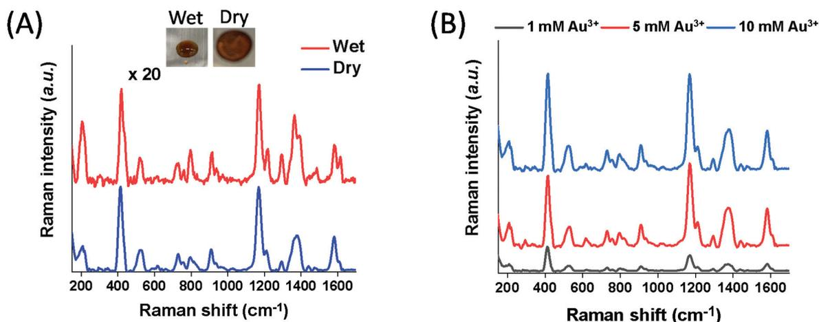
Fig. 4 (A) Comparison of the SERS spectra of 2  $\mu\text{M}$  MGITC under wet and dry conditions using 10 mM Au@Fe<sub>3</sub>O<sub>4</sub>@BCNCs. Inset pictures show before/after drying of 10  $\mu\text{L}$  of the droplet including the nanocomposites. (B) The SERS spectra of 2  $\mu\text{M}$  MGITC using the Au@Fe<sub>3</sub>O<sub>4</sub>@BCNCs with different Au coating condition (1, 5, and 10 mM Au<sup>3+</sup>). All spectra shown here are the average of 400 collected spectra.
