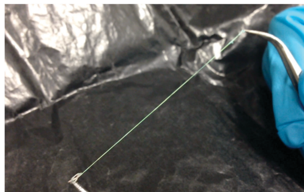
Fig. 8 A long ( \sim 20\text{ cm} ) sample of a PI fibre filled with a mixture of 25% w/w ZLI-3786 in RO-TN 651, viewed under ambient room lighting.
