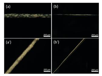
Samples of thicker PI fibres spun from 14% PI in n-hexane dope and filled with RO-TN 615. Scale bars 200 µm. Bottom images correspond to the upper images, with the sample rotated by 45° counterclockwise, showing a substantial brightening when the fibre no longer lies along either of the polariser axes. Both (a) and (b) represent different fibre samples without stretching
