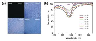
Fig. 3 (a) The polarized optical microscopy images of the coating after illuminating with 365 nm light from 0 to 10 minutes. (b) The temperaturedependent transmission spectra of the stratified coating containing S1011 as the chiral dopant on polycarbonate foil.
