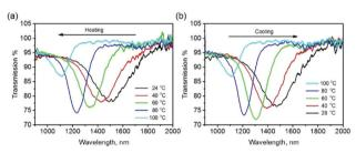
Fig. 5 The transmission spectra of a stratified coating containing a temperature-responsive chiral dopant on the polycarbonate foil upon (a) heating and (b) cooling.
