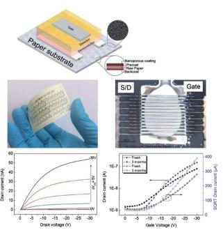
Fig. 6 Fully inkjet-printed polymer TFTs fabricated by Mitra et al. on commercially available specialty paper (p\_e:smart; Felix Schoeller Group). All TFT layers (source/drain contacts, semiconductor, gate dielectric, gate electrodes) were deposited by inkjet printing. Reprinted with permission.<sup>42</sup> Copyright 2017, Wiley-VCH.
