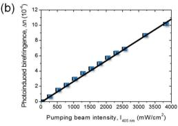
Fig. 3 Dependence of measured photoinduced birefringence on power excitation intensity from the pump beam (long-term photo-ordering). (a) Switching behaviour. (b) Dependence of the photoinduced refractive index anisotropy (birefringence),  $\Delta n$ , on the pumping beam intensity.
