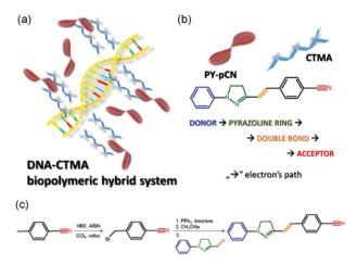
(a) Scheme of the photoisomerizable dye semi-intercalation in the DNA-CTMA matrix. (b) Chemical structure of the photoactive medium (PY-pCN). Arrows in the schematics indicate intramolecular charge transfer paths for electrons. (c) Steps of PY-pCN synthesis. NBS: N-bromosuccinimide; AIBN: azobisisobutyronitrile; PPh<sub>3</sub>: triphenylphosphane.
