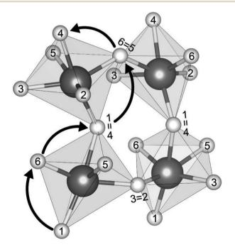
Fig. 2 Connectivity between octahedra in distorted anti-perovskites. Atomic sites of mobile ions are numbered; identical sites in different octahedra adopt the same number. (Selected shared vertex sites are indicated with an equals sign.) Arrows illustrate an example of a migration pathway resulting in long-range ion transport.
