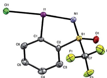
Fig. 2 Structure of (S)-(–)-chloriodane, **9**, as determined by X-ray diffraction. Selected bond lengths and angles: I1–Cl1: 2.576(2) Å; I1–N1: 2.102(6) Å; N1–S1: 1.498(8) Å; angle: Cl1–I1–N1: 174.9(2)°; C1–I1–Cl1: 89.5(2)°; C1–I1–N1: 85.4(3)°; torsion: C6–C1–I1–Cl1: 5.1(7)°; C2–C1–I1–N1: 3.3(6)°. H atoms are omitted for clarity; thermal ellipsoids given at 50% probability.
