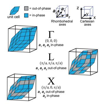
Fig. 3 The translational symmetry, in real space, of the high-symmetry **k** points ( $\Gamma$ , L & X) for the double-perovskite structure.
