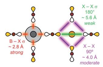
Fig. 6 Hierarchy of bonding interactions in a halide perovskite lattice. Distances are given for  $Cs_2AgBiBr_6$ .<sup>10</sup> B = metal, X = Cl, Br or I.
