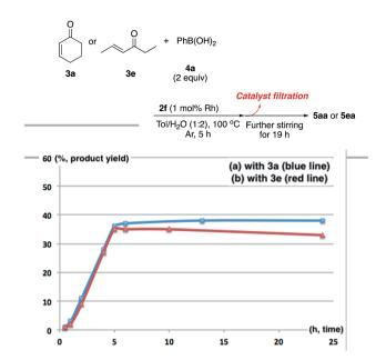
Fig. 1 Hot filtration test.
