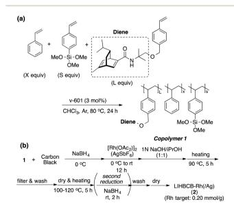
Scheme 2 Preparation of chiral polymer and catalyst.
