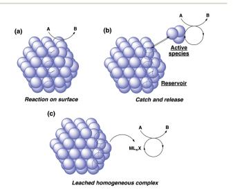
**Scheme 3** Possible mechanisms of heterogeneous metal nanoparticle catalysts.
