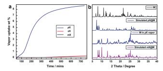
Fig. 5 Vapor sorption of M. (a) Kinetics of pX (blue), mX (black), oX (red) vapour sorption for M at 298 K, respectively. (b) The PXRD of M in pX vapor sorption sample is most consistent with the mX@M in liquid.
