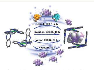
Fig. 1 Schematic illustration of the adsorption behavior of the non-porous molecular crystal M. M readily forms host–guest complexes upon exposure to xylene isomers in liquid, vapor or solution phases and can be recovered upon exposure to vacuum drying.
