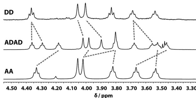
Fig. 6 Aliphatic region of the  $^1\text{H}$  NMR ( $\text{CDCl}_3$ , 298 K) spectra of DD (400 MHz, 1 mM), ADAD (500 MHz, 5 mM), and AA (400 MHz, 5 mM). Chemically related signals are connected with dashed lines.
