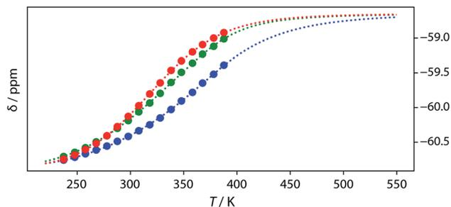
Fig. 11  $^{19}\text{F}$  NMR (500 MHz,  $\text{TCE-d}_2$ , 7.4 mM) melting experiments. The lines show fitting of a two-state equilibrium isochore to the AD data (red) and a three-state equilibrium isochore to the ADAD data (inner residue green, outer residue blue).
