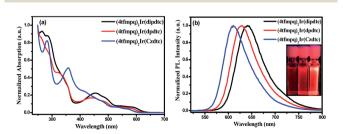
Fig. 3 The UV-vis absorption (a) and emission (b) spectra of the three complexes  $(4tfmpq)_2Ir(dipdtc)$ ,  $(4tfmpq)_2Ir(dpdtc)$  and  $(4tfmpq)_2-Ir(Czdtc)$  in degassed dichloromethane  $(5\times10^{-5}\ \text{M})$  at room temperature.
