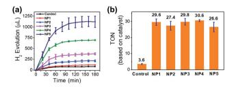
Fig. 5 (a) Photocatalytic H<sub>2</sub> evolution and (b) TON based on FeFe-COOH moieties for NP1-NP5, with free FeFe-COOH as a control. The concentration of incorporated FeFe-COOH was 9.0, 17.7, 28.2, 50.7 and 93.6  $\mu$ M, respectively. The optical power was 200 mW cm<sup>-2</sup>.
