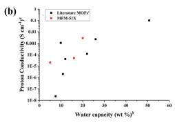
Fig. 6 (a) Adsorption isotherms for water in MFM-510, -511, and -512. Desorption isotherms are shown in ESI† for clarity. (b) Relationship between water capacity and proton conductivity for MFM-510, -511, and -512 and a selection of MOFs in literature. <sup>a</sup>Impedance measurements at high humidity and room temperature, full details in Table S4.† <sup>b</sup>Water capacity at the RH of the impedance data. <sup>c</sup>Water uptake assessed by volumetric or gravimetric analysis.
