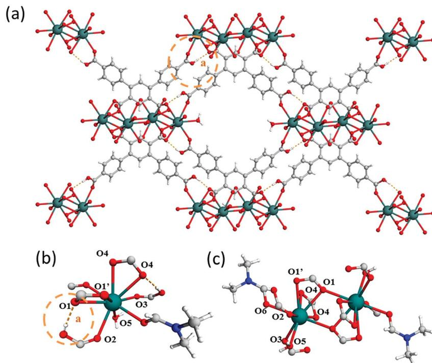
Fig. 3 View of (a) the crystal structure in MFM-511 along the *a*-axis, highlighting restrictive hydrogen bonding of carboxyl proton ( $a = 1.79 \text{ \AA}$ ); (b) the Ba(II) metal node in MFM-511 showing monocapped square antiprismatic coordinate geometry; (c) the binuclear Ba(II) moiety in MFM-511 viewed along the *a*-axis. Carbon, grey; oxygen, red; hydrogen, white; nitrogen, blue; barium, teal.
