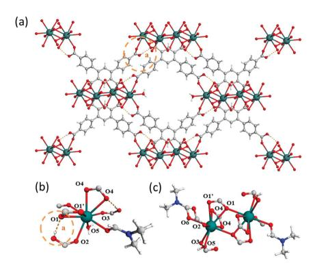
Fig. 3 View of (a) the crystal structure in MFM-511 along the a-axis, highlighting restrictive hydrogen bonding of carboxyl proton (a = 1.79 Å); (b) the Ba(II) metal node in MFM-511 showing monocapped square antiprismatic coordinate geometry; (c) the binuclear Ba(II) moiety in MFM-511 viewed along the a-axis. Carbon, grey; oxygen, red; hydrogen, white; nitrogen, blue; barium, teal.
