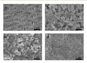
Fig. 2 SEM images of (a) PP separator film, (b) Al<sub>2</sub>O<sub>3</sub> layer on the surface of PP separator film, (c) LAGP layer on PP separator film, (d) PVDF-HFP layer on PP separator film.
