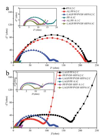
Fig. 6 AC impedance spectra for the NCM811/Li half-cells before and after 100 cycles at 0.2C.
