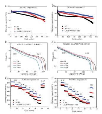
Fig. 8 Charge-discharge cycling of (a) NCM811||Li cells at 0.2C; and (b) NCM811||C cells at 0.2C. Discharge profiles of (c) NCM811||Li cell with LAGP/PP/PVDF-HFP separators film; and (d) NCM811||C cell with LAGP/PP/PVDF-HFP separators film. Rate performance of (e) NCM811||Li cells and (f) NCM811||C cells.
