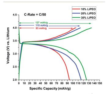
Fig. 3 Effect of salt concentration in PEO electrolyte on  $2^{nd}$  cycle of charge discharge of LiFePO<sub>4</sub> half cells at 60 °C.
