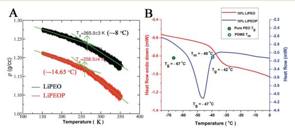
Fig. 5 The theoretical (A) and experimental (B) DSC curves of LiPEO and LiPEOP. The  $T_g$  of the pure PEO (the reported value) is denoted by the green dot in the (B). The sky blue dot in the figure is the  $T_m$  of the PDMS.
