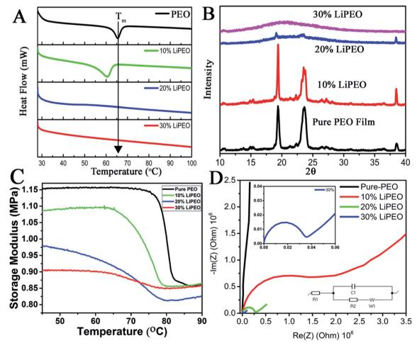
Fig. 1 (A) DSC plots and (B) XRD patterns of different SEs. (C) Storage modulus (MPa) vs. temperature (°C) curves at a frequency of 1 Hz.  $^*T_m$  is assigned to the minima of derivative of the sigmoid curves. (D) The EIS (Nyquist plots) of different samples. The simulated Randles circuit which fit the spectra is also shown in the inset.
