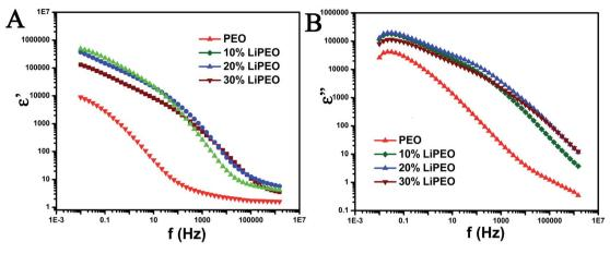
Fig. 2 (A)  $\varepsilon'$  vs. frequency (f in Hz) and (B)  $\varepsilon''$  vs. frequency plot for different samples. The scales are in log.
