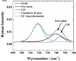
Fig. 3 Deconvolution of S-N-S stretching vibrational mode of the TFSI-anion: (a) in liquid electrolyte, (b) in PGPE.
