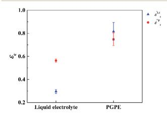
Fig. 7 Effective charges for Li (blue triangles) and TFSI (red circles) at  $20\,^{\circ}\text{C}$  measured by  $^{7}\text{Li}$  and  $^{19}\text{F}$  NMR respectively. Errors are calculated by error propagation.
