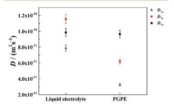
Fig. 4 Self-diffusion coefficients of PGPE and liquid electrolyte: Li (blue triangles), TFSA (red circles) and BOB (black squares) at 25  $^{\circ}$ C measured by  $^{7}$ Li,  $^{19}$ F and  $^{13}$ C PFG-NMR, respectively. Errors are calculated by error propagation.
