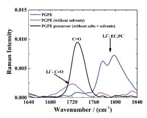
Fig. 5 Raman spectra of C=O stretching mode of PMMA by introducing the same salts and solvents as in PGPE.
