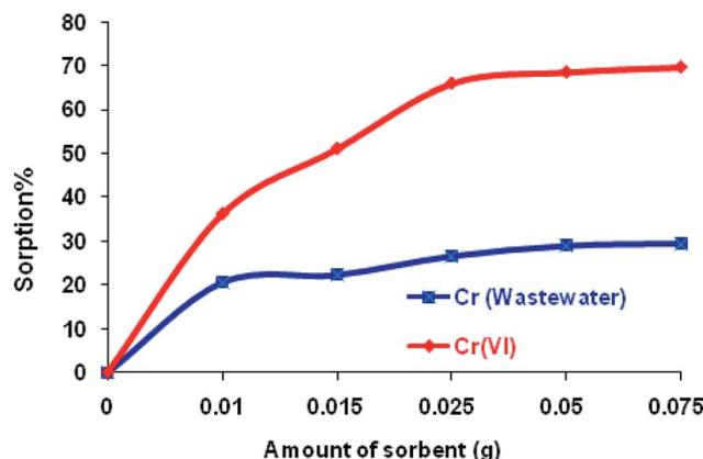
Fig. 8 The effect of the amount of sorbent on the sorption of Cr(vi) from aqueous solution and wastewater.
