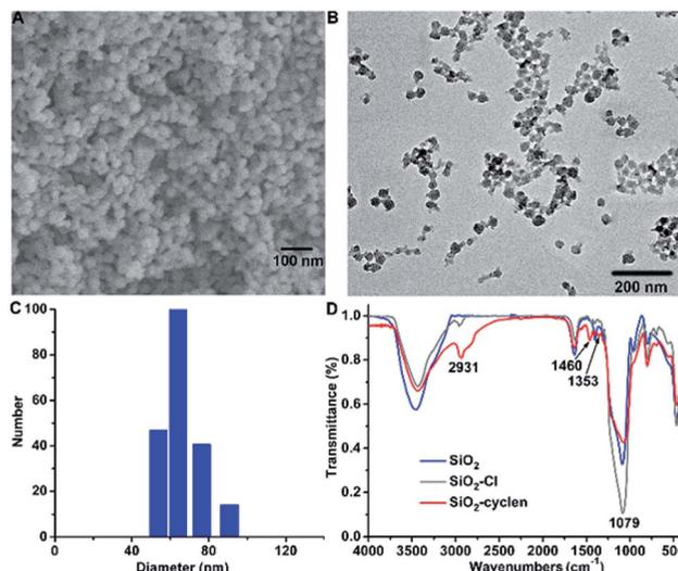
Fig. 1 SEM image (A), TEM image (B), DLS size distribution (C) of SiO<sub>2</sub>-cyclen nano-chelator, and FT-IR spectra (KBr) of SiO<sub>2</sub>, SiO<sub>2</sub>-Cl and SiO<sub>2</sub>-cyclen (D).
