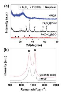
Fig. 2 (a) XRD patterns of the Fe(OH) $_3$ @GO hybrid film, Fe $_3$ O $_4$ @rGO hybrid film and HWGF, and (b) Raman spectra of the HWGF and the graphite oxide.
