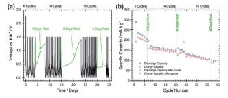
Fig. 4 (a) Voltage profile of a pause test at 25 mA g $^{-1}$  using BMG as the working electrode. Potential limitations of 0.01 V and 1.5 V vs. K/K $^+$  were used with the following cycling regime: 6 cycles, rest 4 days, 14 cycles, rest 8 days, 16 cycles, rest 4 days, continued cycling. (b) Specific capacity for galvanostatic discharge/charge cycles during the pause test
