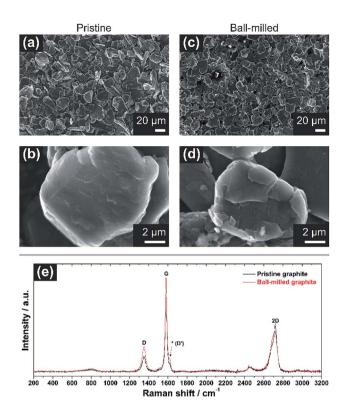
Fig. 1 (a and b) SEM images of the pristine graphite (PG) electrode at low  $(1000\times)$  and high  $(20\ 000\times)$  magnification. (c and d) SEM micrographs of ball-milled graphite (BMG) electrode at low and high magnification. (e) Normalized Raman spectra of pristine (black) and ball-milled graphite (red). Note the increase of the relative intensity of the 'D' band in (e) after ball-milling, as well as a more prominent signal at  $\sim 1620\ \text{cm}^{-1}$  (see asterisk).
