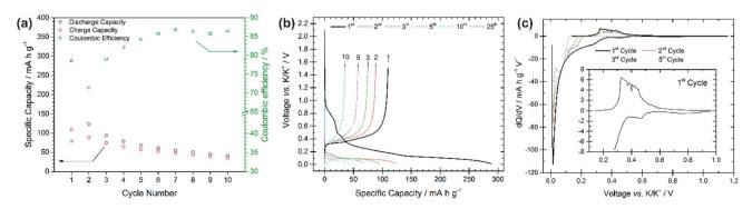
Fig. 2 (a) Specific capacity vs. cycle number for the pristine graphite electrode galvanostatically cycled at 25 mA  $g^{-1}$  with potential limitations of 0.01 V and 1.5 V vs. K/K<sup>+</sup>. (b) Voltage profiles vs. specific capacity for selected cycle numbers from the same test. (c) dQ/dV plots for cycles 1, 2, 3 and 5 for the same test.
