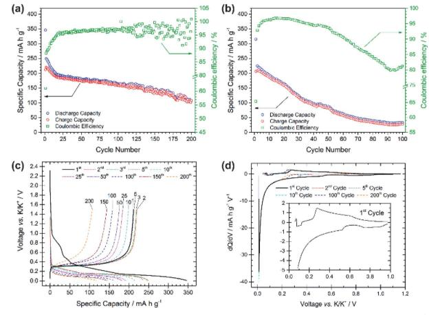
Fig. 3 Specific capacity vs. cycle number for the ball-milled graphite (BMG) electrode galvanostatically cycled at (a)  $25 \text{ mA g}^{-1}$  and (b) 250 mA  $g^{-1}$  with potential limitations of 0.01 V and 1.5 V vs. K/K<sup>+</sup>. (c) Voltage profiles vs. specific capacity for selected cycle numbers from the test at 25 mA  $g^{-1}$ . (d) dQ/dV plots for cycles 1, 2, 5, 10, 100, and 200 from the test at 25 mA  $g^{-1}$ .
