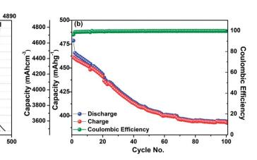
Fig. 3 (a) The cyclic galvanostatic discharge-charge profiles for  $Bi-LiBH_4-AB$  composite electrodes in the voltage range of 0.2-1.5 V at 0.1C. Only selected cycles (1, 5, 10, 20, 30, 40, 50, 60, 70, 80, 90, 100) are shown for clear visibility. (b) Cyclic stability of Bi−LiBH₄-AB composite electrodes as shown by discharge/charge capacity and the coulombic efficiency vs. cycle no.
