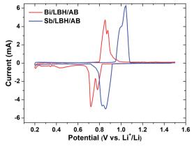
Fig. 1 Cyclic voltammograms of Bi and Sb composite electrode scanned at  $0.1 \, \mathrm{mV \ s^{-1}}$ .
