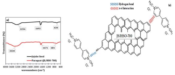
Fig. 8 (a) FTIR spectra of JS/HSO-700 after paraguat adsorption; (b) proposed adsorption mechanism of paraguat onto JS/HSO-700.
