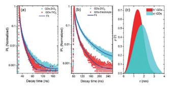
Fig. 4 Comparison of the transient PL curves of heterostructured QDs: (a) deposited onto a ZrO2 and TiO2 mesoporous film; (b) deposited onto a ZrO2 mesoporous film and QDs with electrolyte. The excitation wavelength is  $\lambda_{ex}$  = 444 nm. (c) Comparison of the spatial probability distribution value  $\rho(r)$  of the electron and hole as a function of QD radius r (nm) (H = 2.15 nm, red for hole and cyan for an electron).
