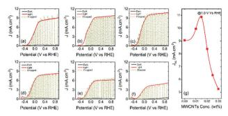
Fig. 5 Photocurrent density-potential curves of PEC devices based on colloidal heterostructured QD sensitized TiO2-MWCNTs hybrid photoanodes with different concentrations of MWCNTs under dark, continuous and chopped illumination (AM 1.5G, 100 mW cm<sup>-2</sup>): (a) 0.0 wt%; (b) 0.010 wt%; (c) 0.015 wt%; (d) 0.020 wt%; (e) 0.025 wt% and (f) 0.030 wt%. (g) Variation of current density at 1.0 V vs. RHE under 100 mW cm<sup>-2</sup> illumination with the concentration of MWCNTs.
