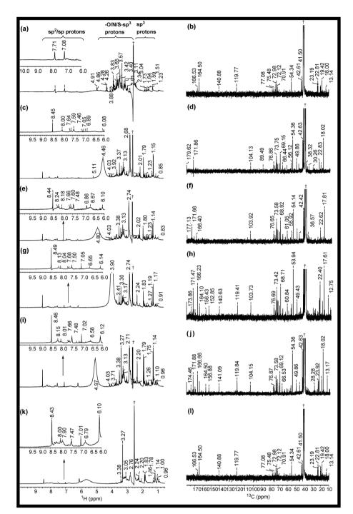
Fig. 2  $^{1}$ H,  $^{13}$ C (1D) NMR spectra of (a, b) RE, (c, d) NSR-1 h, (e, f) NSR-2 h, (g, h) NSR-3 h, (i, j) NSR-4 h intermediates and (k, l) N-S@RCD. The spectra were recorded in dimethyl sulfoxide-d<sub>6</sub> solvent and  $\delta = 2.50$  and 39.50 ppm were considered as reference peaks.  $^{\dagger}$ Peak for the dimethyl sulfoxide-d<sub>6</sub> solvent.
