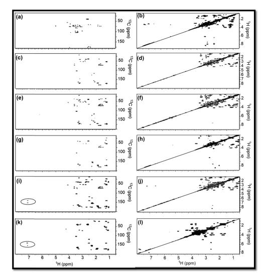
Fig. 3 HMBC, COSY NMR (2D) spectra of (a, b) RE, (c, d) NSR-1 h, (e, f) NSR-2 h, (g, h) NSR-3 h, (i, j) NSR-4 h intermediates and (k, l) N-S@RCD. The spectra were recorded in dimethyl sulfoxide- $d_6$  solvent and the  $\delta$  ( $^{13}$ C/ $^{1}$ H) = 39.50/2.50 ppm is considered as a reference signal.
