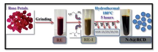
Scheme 1 Schematic for synthesis of N-S@RCD and intermediates.
