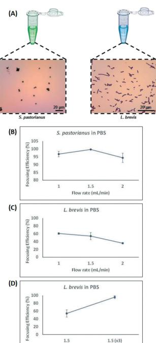
Fig. 2 Optimisation of separation for S. pastorianus and L. brevis. A) Micrographs of gram-stained S. pastorianus and I. brevis cells B) Results for flow rate optimization of S. pastorianus separation using cell counts and L. brevis based on OD measurements (C and D). The optimal fractionation was found to occur at 1.5 mL per min for S. pastorianus and L. brevis. All values were analysed in biological triplicate.
