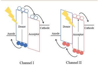
Fig. 1 Channel I and II excitation in organic solar cells.
