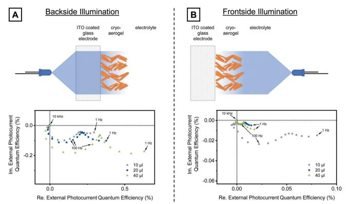
Fig. 5 IMPS responses of cryoaerogel coated photoelectrodes with different film thicknesses. For the preparation of all samples, a 28 mM NPL solution dispersed in  $1 \times 10^{-2}$  M KOH was applied. The samples were irradiated either from the backside (A) or from the frontside (B). The sketches (top) illustrate the differences between both types of irradiation. All IMPS spectra (bottom) were measured at a bias potential of 300 mV.
