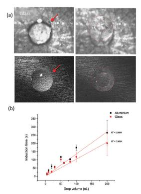
Fig. 5 (a) Images of 100 nL droplets on glass and aluminium foil substrates with the red arrow indicating the point of start of crystallisation and red dotted-line circles indicating coffee-ring formation during droplet drying, and (b) crystallisation induction time as a function of drop volume in droplets printed on both substrates.
