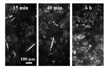
**Fig. 2** Online images recorded during the seeded crystallization of form II with the following operating conditions: T=0 °C,  $c_0^{\rm liq}=300$  mg  $g_{\rm EtOH}^{-1}$ , N=400 rpm.
