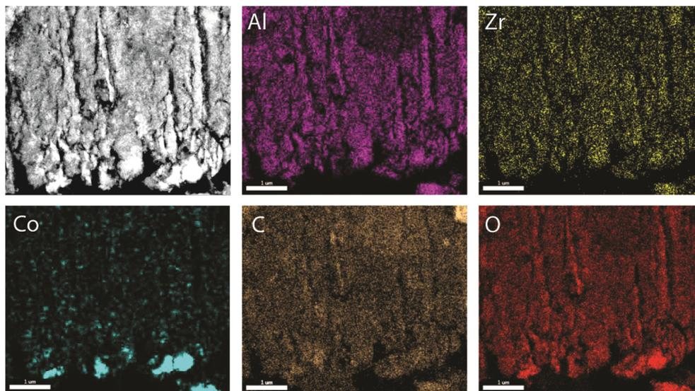
Fig. 4 Representative HAADF-STEM micrograph (top-left panel) of an ultramicrotomed cross section (150 nm nominal thickness) of a Co/CNT-ZrAlO<sub>x</sub> micromonolithic catalyst and EDX compositional maps of the same region obtained from the corresponding K-spectral lines.
