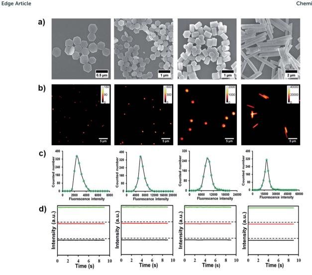
Fig. 1 (a and b) are the SEM and single-particle fluorescence microscopy images of UCNPs-1, -2, -3 and -4. (c) Fluorescence intensity distribution histograms of the corresponding UCNPs. (d) Representative single-particle fluorescence intensity tracks as a function of time in (b).
