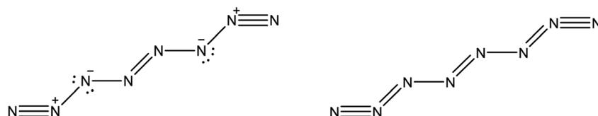
Fig. 5 Lewis structure of the  $\text{N}_8$  molecule. On the left, the structure depicted by Hirshberg *et al.* in their 2014 paper, obtained through NBO and bond length analysis. On the right, the structure suggested by DI analysis.
