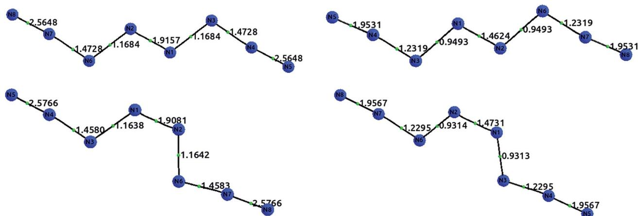
Fig. 6 Optimized structures with delocalization indices displayed for the isomers EEE (top) and EZE (bottom) of the  $N_8$  molecule. The left diagrams show the HF values, and the right diagrams the CCSD values.
