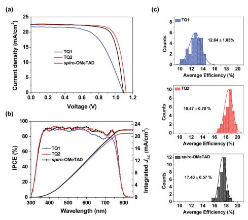
Fig. 4 (a) The J-V curves for the best-performing devices using TQ1, TQ2, and spiro-OMeTAD as HTMs. (b) IPCE spectra of the solar cell devices based on different HTMs. (c) Statistical distribution in efficiencies of the perovskite solar cells fabricated with TQ1, TQ2, and spiro-OMeTAD as the HTM, respectively.
