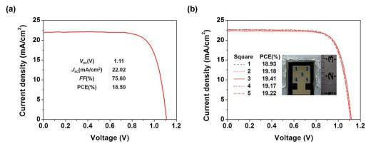
Fig. 7 (a) The J-V curves for the optimized large area (1.02 cm<sup>2</sup>) devices using TQ2 as the HTM. (b) J-V curves measured from five different spots with an aperture area of 0.09 cm<sup>2</sup> selected from the large area device.
