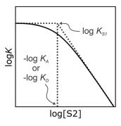
Fig. 2 Dependence of the association constant (log K) for formation of a 1:1 complex between a H-bond donor and acceptor on the concentration of a polar solvent (S2) in a non-polar solvent (S1). log  $K_{\rm S1}$  is the D·A association constant in pure S1, and log  $K_{\rm D}$  and log  $K_{\rm A}$  are the D·S2 and A·S2 association constants in pure S1.
