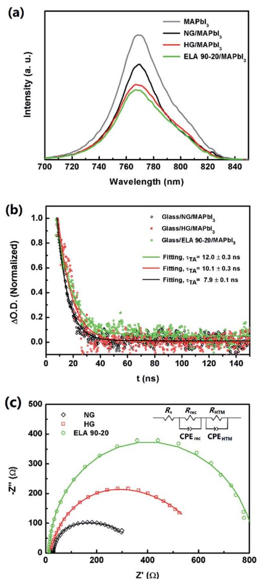
Fig. 7 (a) PL spectra of glass substrate/ETL/MAPbI<sub>3</sub> (ETL = NG, HG, ETL 90-20, or none) samples. (b) Transient absorption decay of glass substrate/ETL/MAPbI<sub>3</sub> (ETL = NG, HG, and ETL 90-20) samples. (c) Nyquist plots of the PHJ-PSCs based on NG, HG, and ELA 90-20. The inset is the equivalent circuit of the cell.
