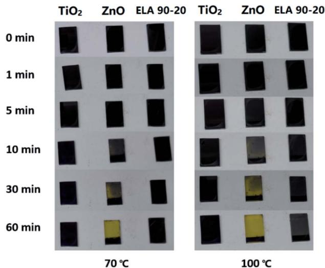
Fig. 8 Photographs of MAPbI<sub>3</sub> films deposited on different samples (TiO<sub>2</sub>, HZ and ELA 90-20 films) and heated to either 70 °C or 100 °C for the indicated time.
