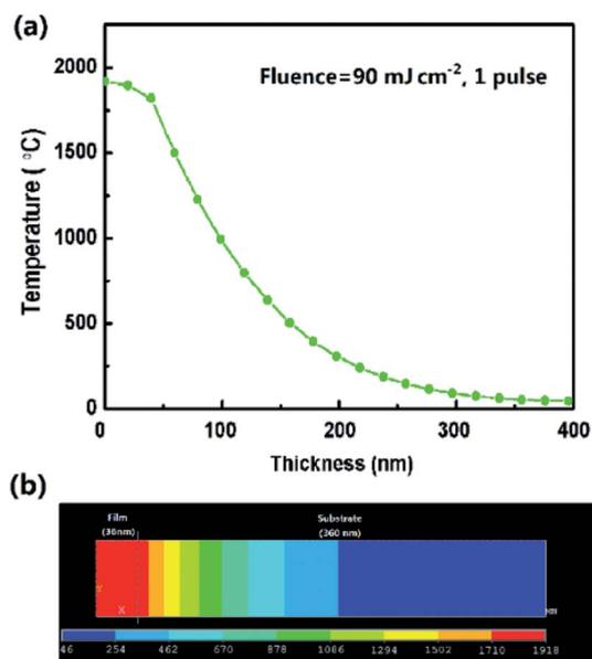
Fig. 4 (a) Temperature distribution along the film thickness when loading fluence of  $90 \text{ mJ cm}^{-2}$  for 1 pulse (20 ns). (b) Temperature distribution in two dimensions model of ELA 90-20 at 20 ns.
