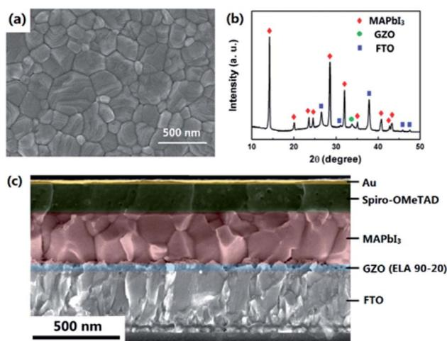
Fig. 5 (a) SEM image of MAPbI<sub>3</sub> layer on ELA 90-20. (b) XRD pattern of the MAPbI<sub>3</sub> film prepared on the ELA 90-20 at FTO substrate. (c) Cross-sectional SEM image of the cell employing ELA 90-20.
