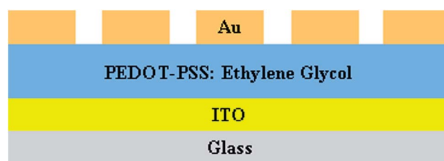
Fig. 3 Schematic representation of the sensor device on ITO-coated glass.
