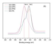
Fig. 10  $\,$  O 1s (a) and N 1s (b) high resolution XPS spectra of GO, GO-DBA, GO-DPA, GO-PPD and GO-PA.
