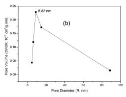
Fig. 3 N<sub>2</sub> adsorption-desorption isotherm for GO: (a) BET surface area measurement and (b) BJH pore size distribution.
