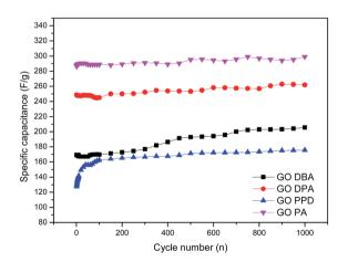
Fig. 13 Cyclic stability tests for the amine-functionalized electrodes at 1 mA  $\rm cm^{-2}$  discharge current density in aqueous 1.0 M  $\rm H_2SO_4$  electrolyte solution.
