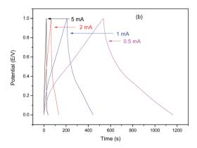
Fig. 12 Galvanostatic charge–discharge curves in 1.0 M  $\rm H_2SO_4$  for (a) GO and amine-functionalized GO at 1.0 mA cm $^{-2}$  and for (b) GO-DPA at different current densities.
