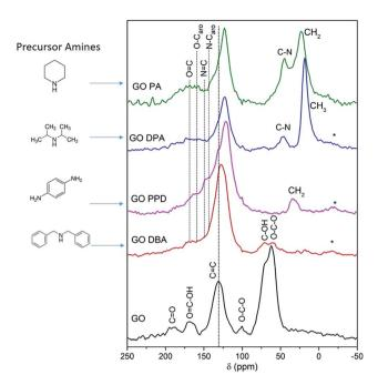
Fig. 7  $\,^{13}\mathrm{C}$  NMR spectra of GO and GO-amines. The asterisks indicate spinning sidebands.
