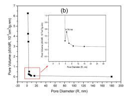
Fig. 4 N<sub>2</sub> adsorption-desorption isotherm for GO-DBA: (a) BET surface area measurement and (b) BJH pore size distribution.
