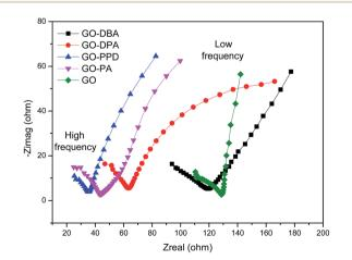
Fig. 14 Electrochemical impedance spectroscopy (EIS) of GO and the amine-functionalized electrodes in aqueous 1.0 M  $\rm H_2SO_4$  electrolyte solution.
