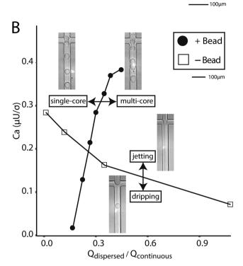
Fig. 4 Bead-dependent drop formation in the jetting regime without an aqueous co-flow. A) Microscope images of single-bead and multibead containing drops. B) Phase diagram of the transition from single-to multi-bead drops as a function of capillary number and flow rate ratio. Images of devices depict operation in particular regions.
