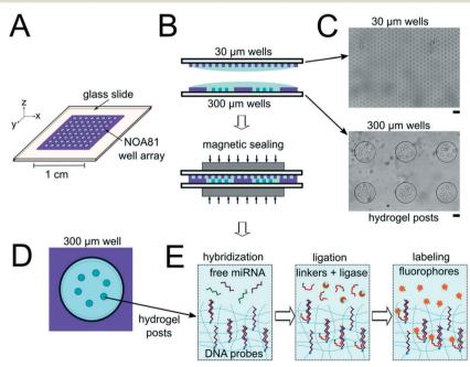
Fig. 1 Device and assay overview. (A) Well array on glass slide schematic. (B) Side view of the isolated reactor formation using nanoliter well arrays. (C) Bright field images of the top (30 µm wells) and bottom (300 µm wells) arrays. (D) Schematic of well in the array containing PEDGA posts functionalized with DNA probes complimentary to miRNA targets. (E) Hybridization and ligation-based miRNA detection assay schematic. Scale bars are 100 um.
