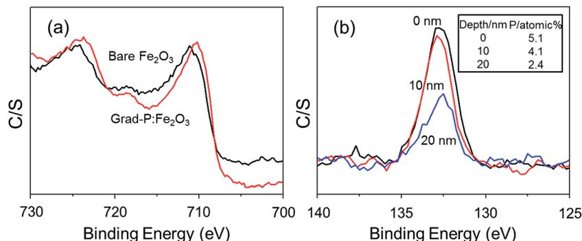
Fig. 3 (a) XPS spectra of the Fe 2p signal in bare  $\text{Fe}_2\text{O}_3$  and grad-P: $\text{Fe}_2\text{O}_3$  photoanodes; (b) XPS depth profile signal of P 2p in grad-P: $\text{Fe}_2\text{O}_3$ , where the P concentration decreases with increasing sputtering time (inset shows the P atomic concentration values at different depth).
