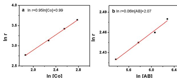
Fig. 4 (a) The plot of hydrogen generation rate *versus* the concentration of Co both in natural logarithmic scale,  $\ln(\text{rate}) = 0.95 \ln[\text{Co}] + 0.99$ ; (b) the plot of hydrogen generation rate *versus* the concentration of AB both in natural logarithmic scale,  $\ln(\text{rate}) = 0.06 \ln[\text{AB}] + 2.07$ .
