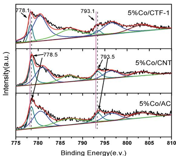
Fig. 6 XPS spectra of Co 2p<sub>3/2</sub> and 2p<sub>1/2</sub> in 5% Co/CTF-1, 5% Co/CNT and 5% Co/AC samples. All samples were pre-treated with Ar<sup>+</sup> sputtering.
