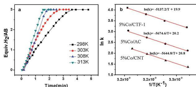
Fig. 7 (a) Plots of volume of H<sub>2</sub> vs. time for the 5% Co/CTF-1 catalyzed hydrolysis of AB at temperatures in the range of 298–313 K, catalyst/AB = 0.05; (b) Arrhenius plots obtained from the kinetic data of 5% Co/CTF-1, 5% Co/CNT, and 5% Co/AC.
